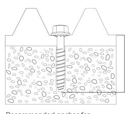
Recommended anchor for installation on concrete or asphalt.
