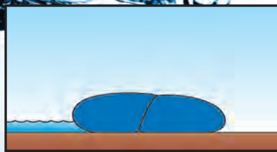
Baffle shifts to stabilize the dam.
