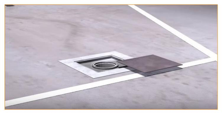
Using a flashlight, complete a visual inspection to evaluate debris accumulation. If the area cannot be fully observed, insert a closedcircuit camera into the system to perform inspection. If accumulation is noted, record the depth of debris. If the debris accumulation is greater than three inches, proceed to maintenance of the Debris Row. If not, record all data and inspection results and close all access lids.
