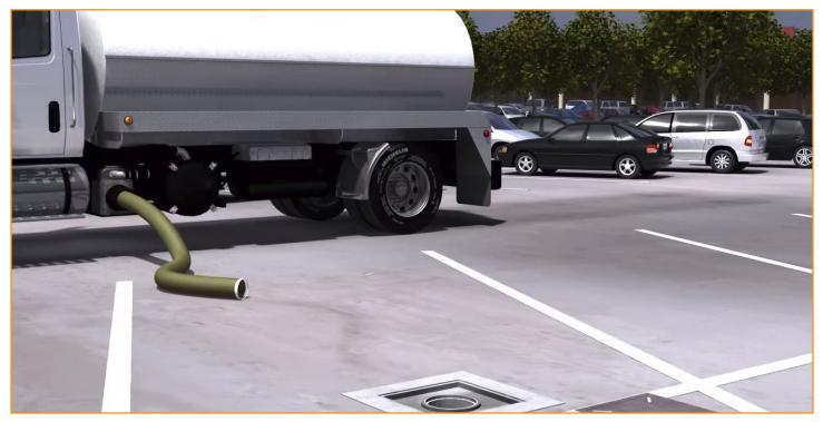
Maintenance is accomplished using a high-pressure nozzle to loosen and suspend debris that can then be removed with a vacuum hose. Once debris has been removed, remove any equipment and close any open ports. Be sure to inspect and vacuum any upslope catch basins and manholes as necessary. Most municipalities and private companies have vacuum equipment with the combined capability to both loosen and remove the accumulated debris.
