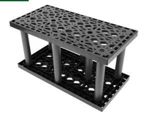
**StormTank™** Stormwater Storage System is a high-void, high strength, affordable alternative to crushed stone, concrete structures, or pipe chambers. Use of StormTank™ reclaims valuable surface space for better surface usage such as recreational areas, parking lots or buildings.
