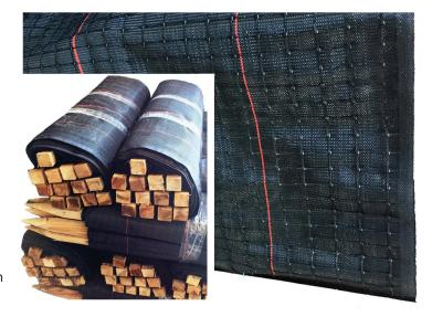
**Installation:** A six inch trench is dug where silt fence is to be placed. The posts are driven into the ground at a depth that allows the first marker line on the fabric to reach the top of the trench, or ground level. This should place the fabric six inches into the ground or trench. Continue to drive all of the posts to the same depth keeping fabric stretched and tight. Back fill the trench with remaining soil.
