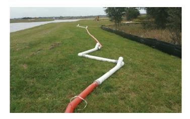
The Link Manifold can be used in a variety of applications that include recirculation to clean turbid water within ponds and for direct discharge when using the appropriate filters to collect flocculated particles created by the manifold sytem.
