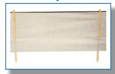
BSRF Priority 2 black band medium-duty silt fence is available in 36" wide nonwoven spunbonded polyester fabic. The system utilizes wood stakes and a specific method of attachment. The fabric, when installed as specified, produces a proven system with superior filtering capabilities in slurry conditions. The system shall be used as a vertical interceptor of sediment transported by overland flow on construction sites.
