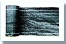
In addition to the D.O.T. silt fence available, we also offer a wire-backed option. A 14 gauge wire mesh with 2" X 4" openings is attached to D.O.T. grade fabric. The fabric is 36" high with 24" or 36" high wire.
